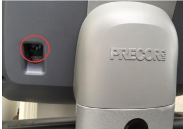
2. **On fitness equipment use a cleaning solution such as rubbing alcohol to clean the area where you would like to attach the GymConnect retrofit module. After cleaning wipe the area dry. Then, clean the bottom of retrofit module and wipe dry and affix the yellow side of the double-sided tape to the bottom of the GymConnect retrofit module.**
