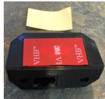
3. **Remove the red side off the double sided tape and attach the GymConnect retrofit module to the fitness equipment device. After securely affixed to the machine, connect the Ethernet cable between the retrofit module and the CSAFE port.**
