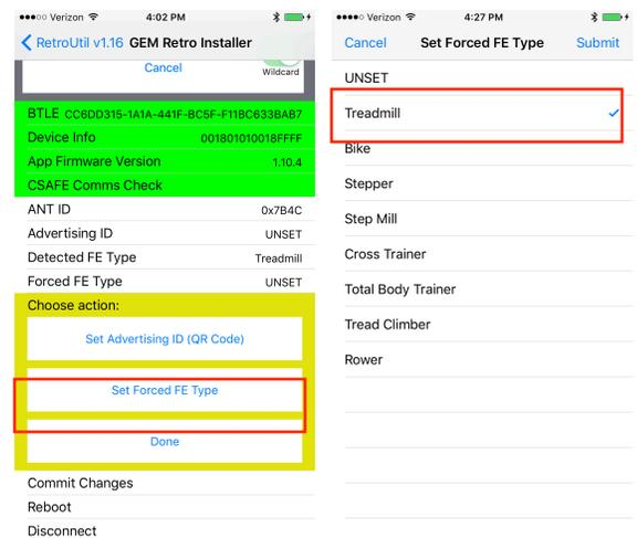
8. After you have configured the Forced FE Type, the set-up is finished. Select done and the RetroUtil app will write the settings in the GymConnect retrofit's memory. The retrofit is now ready to use. Follow the remaining steps below to complete the installation process.
