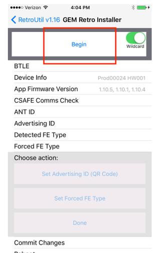
5. On the next screen a list of Retrofit devices that are advertising will appear. Select your device and the RetroUtil app will make a connection to the GymConnect Retrofit. After the app makes the Bluetooth connection to the GymConnect retrofit, the app will check the firmware and update the firmware in the GymConnect Retrofit automatically if it is out of date. Once the firmware update process is completed, you will now be able to configure the retrofit for your equipment.
